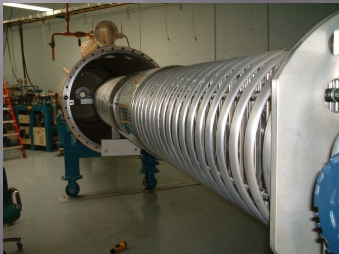
Low-energy end showing ion source and accelerator.
