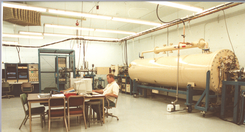
Low-energy end showing ion source and accelerator.
