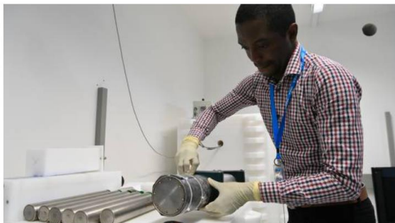
Francois Idjiwole handles a neutron generator at the new IAEA facility in Seibersdorf, Austria. (Photo: D. Calma/IAEA)
