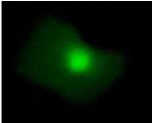
VUV beam visualization on Ce:YAG phosphor
